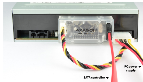
FIGURE 2: Interconnect to ATAPI CD/DVD drive.
